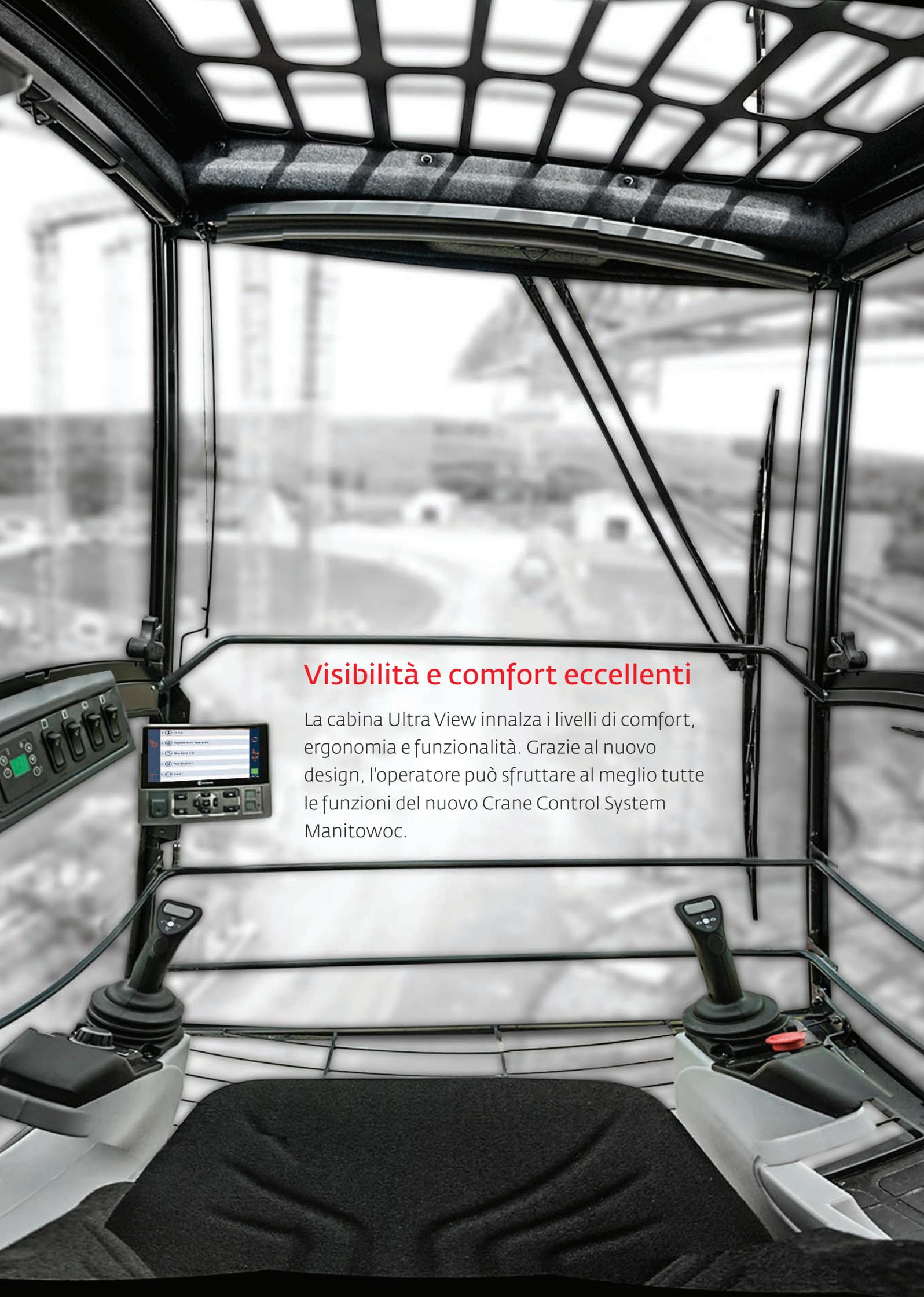
The image shows the interior of a crane cab. At the top, there is a large, grid-patterned skylight. Below it, a wide, clear window provides a view of a blurred outdoor construction site. The cab's interior is equipped with two large joysticks on the operator's seat, a central control panel with a digital display, and various buttons and switches on the left side. The overall design is modern and functional, emphasizing visibility and ergonomics.
